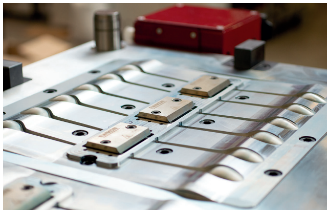
Fig. 2. View of the contour plate on the hot runner side of the mold for the production of the ice-cream spoon. The parts are side gated © Uniform
